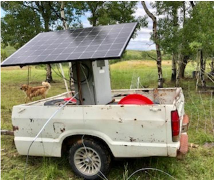
Portable electric fencer
